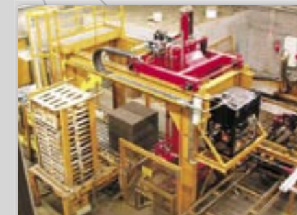
The curing racks are constructed in hot dip galvanised steel profiles.
