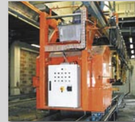
Moulding machine with vibration and overhead travelling vibration roller machine.
