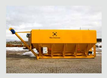
Horizontal hopper in fully welded construction. Complete silo system assembled on a common flat rack hook container. Alternatively the silo can be delivered mounted on a bogie trailer or a flat rack trailer. Designed for easy flowing materials such as Portland cement with a bulk density of 1.13 tonnes/M<sup>3</sup>.
