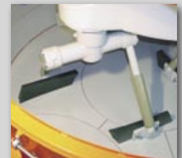
Segmented wear resistant floor and wall linings for easy replacement.
