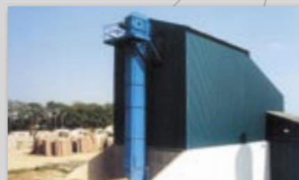
Examples of aggregate bins with an integrated bucket elevator.
