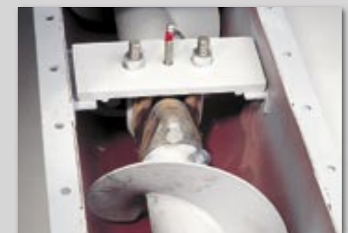
Special intermediate axle bearings used in long conveyors.
