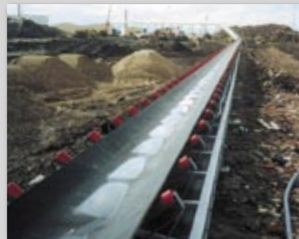
400 t/hr conveying system from loading point to storage supplied to a cement works in Togo, Africa.
