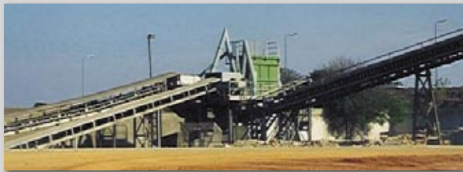
400 t/hr conveying system from loading point to storage supplied to a cement works in Togo, Africa.
