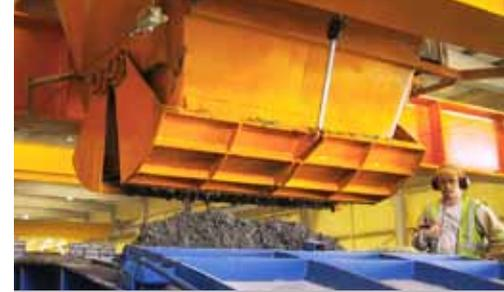
Lightweight concrete spreaders, concrete spreaders for standard concrete and crane systems. Can be combined with a wide range of options.
