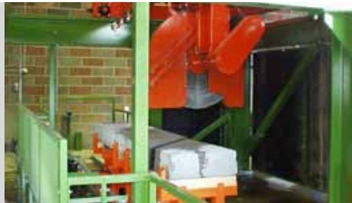
Customised concrete saws for the capping of elements or for the sawing of recesses.
