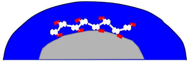
The most recently developed products; the PolyCarboxylate Ethers and Esters additionally work by steric hindrance resulting from the hydrophilic polyether pendent chains which are grafted onto a polyacrylic acid backbone. In total there exists a complex family of PCE products all having influence on rheology, water reduction, workability retention and concrete performance. The user is thus particularly advised to consult the manufacturer before use.
