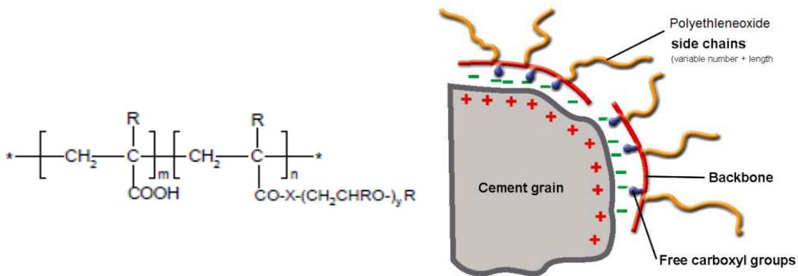
The modes of action of the new Polycarboxylate Ether (PCE) based superplasticiser effects can be observed below:
